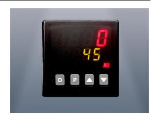
Quick putting into operation: The process-parameters can be established with auto-tune
